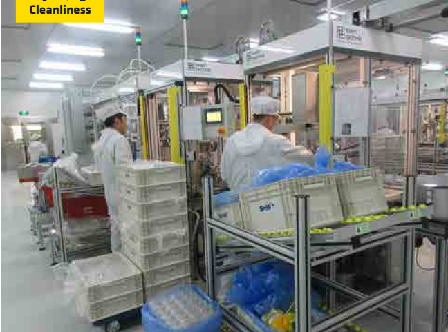
The pumps are washed in the clean room
